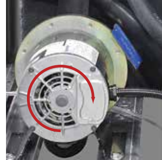
Correct shaft rotation is clockwise.
