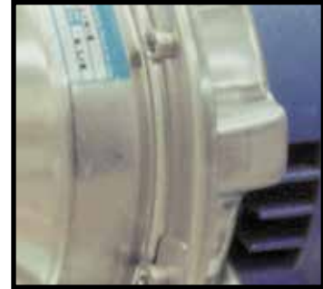
Typical pump casing bolt
