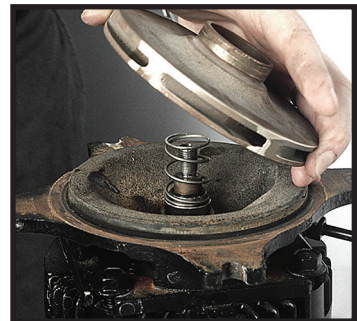
Aligning impeller and spring
