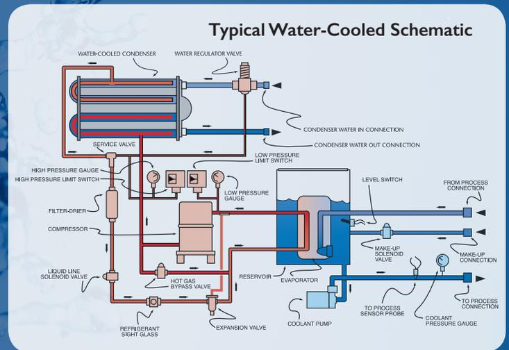
\* Water-cooled models require an external water supply source for operation.
