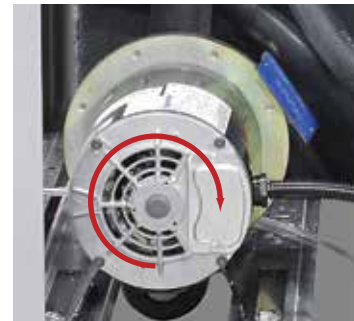
Correct shaft rotation is clockwise.
