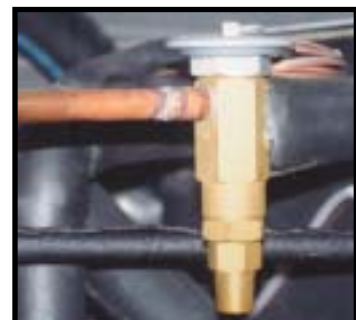
Expansion Valve Figure 6.2F
