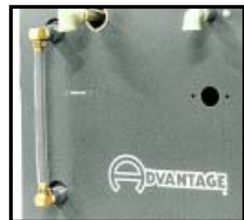
Typical reservoir sight glass Figure 3.2C
