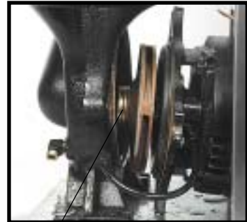
Impeller Figure 5.5E
