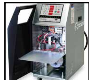
Thermoformed panel removed and electrical cabinet open.
