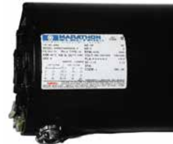
Typical Motor name plate with listed full load amp rating.
