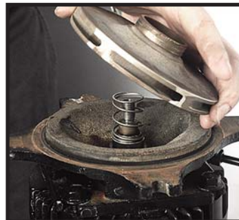
Aligning impeller and spring
