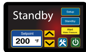
Yellow Alert Icon showing Water Pressure Fault
