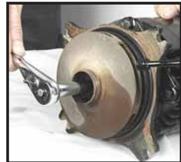
Removing impeller locking screw with ratchet
