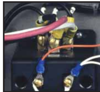
Do not reverse power leads at the unit’s power entry
