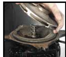
Replacing Impeller Figure 5.5K
